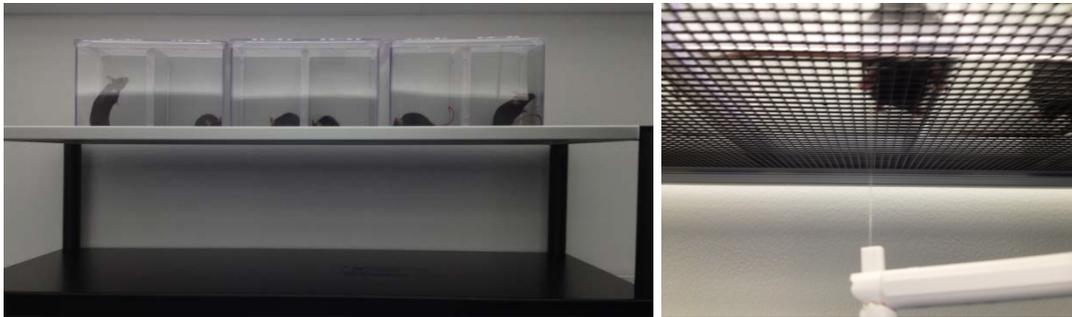
5.1.2. Observation arenas. Clear observation arenas with an open floor that is placed atop the wire floor grid to allow access to the plantar surface of the subject's feet. (Stoelting product # 57823; Multiple Configuration Animal Enclosure for 12 mice with aerated lids; Stoelting Co., Wood Dale, IL, USA; Figure 1)
